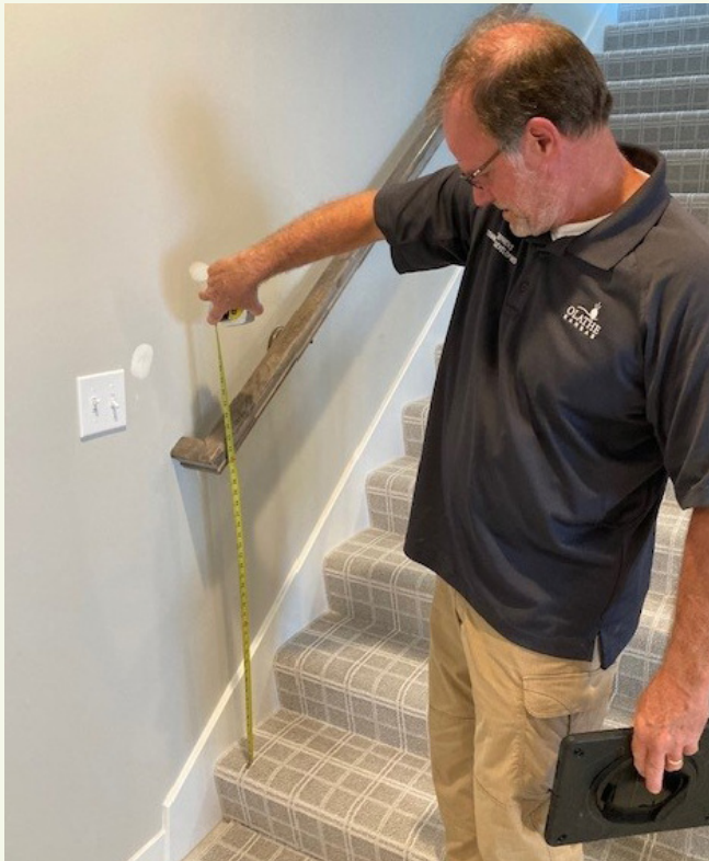
Building Inspector Scott Stephens measures the height of handrails and guardrails on a final residential inspection.
