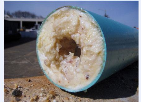
The fats and grease placed down the drain cause backups in sanitary sewer lines.
