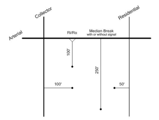
All distances are measured from the edge of pavement to edge of pavement \* Industrial sites may have a driveway throat less than 100'
