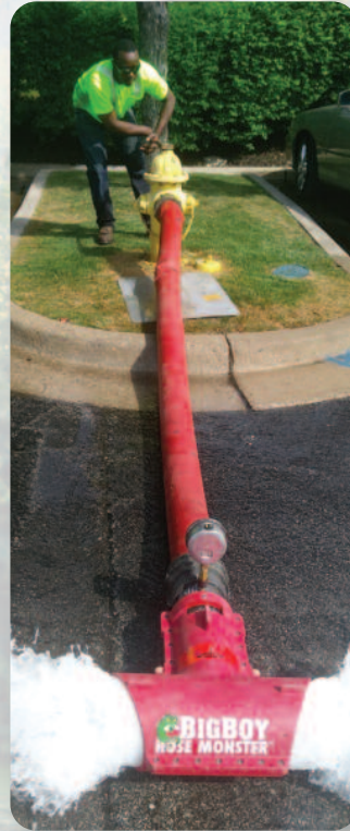
A.J. Brookins, Utility Maintenance, conducts fire hydrant flow testing to help ensure protection of life and property.
