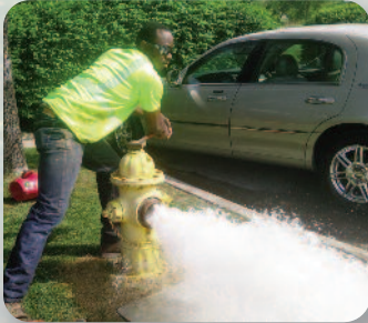
A.J. Brookins, Utility Maintenance, conducts fire hydrant flow testing to help ensure protection of life and property.
