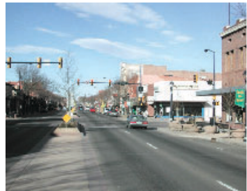
Example of Santa Fe Corridor character with median, curb extensions, street trees, pedestrian lighting, on-street parking, and street furniture
